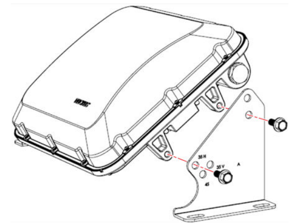
FIGURE 12 Mounting Holes for a 35-Degree Angle
