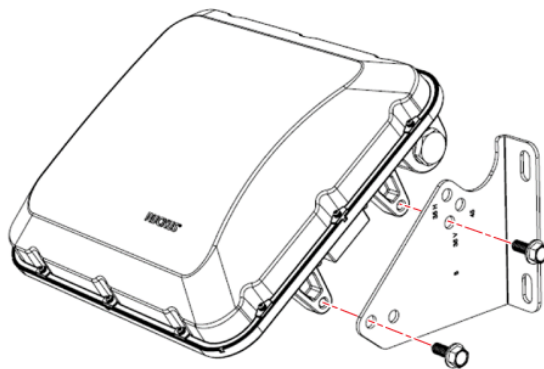
FIGURE 15 Mounting Holes for a 35-Degree Angle
