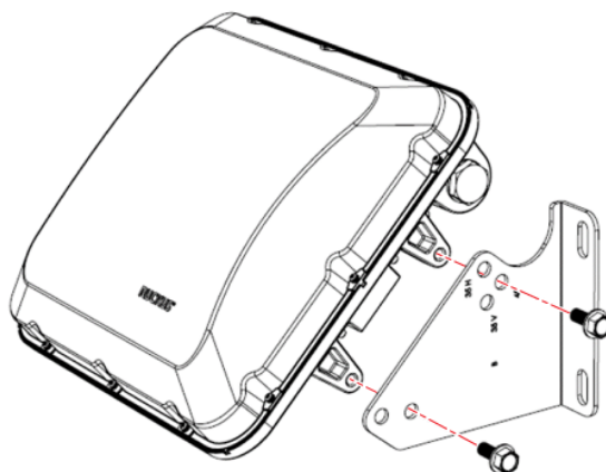
FIGURE 16 Mounting Holes for a 45-Degree Angle
