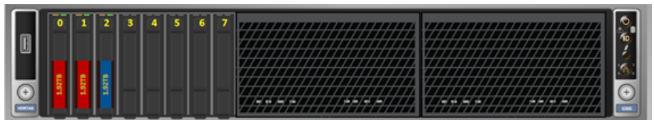
Figure 1-1 Veritas 5350 Appliance front disk drive assignments
