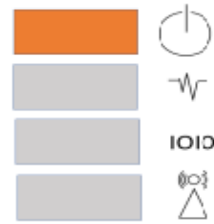
Figure: Power supply does not have redundancy
