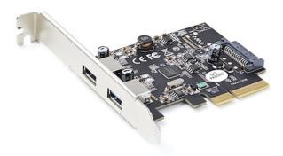
This PCIe USB 3.2 Gen 2 controller card installs into an available PCI-Express x4 slot in your computer and enables you to upgrade your current system by adding two SuperSpeed USB-A (10Gbps) ports.
