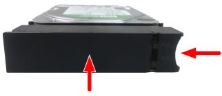
Push in the center to insert the drive carrier into an empty drive bay.
