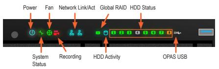
When boot-up is finished, check the LEDs on the front panel to make sure the system is functioning properly.
