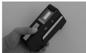
Open the shutter by gripping lever. New cleaning tape will appear.
