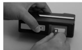
Push and slide a ferrule end face while gripping the lever.
