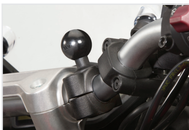
1 RAM-B-408-75-1U RAM® Torque™ Medium Rail Base (pg. 123)
