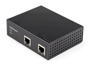
Extends the reach of PoE links up to 328' (100 m) to power powered devices (PD) over long distances; up to 4 extenders can be cascaded to extend the range of a PoE source (PSE) device up to an additional 400m, for a total range of 500m from the original PSE source to the target device.
