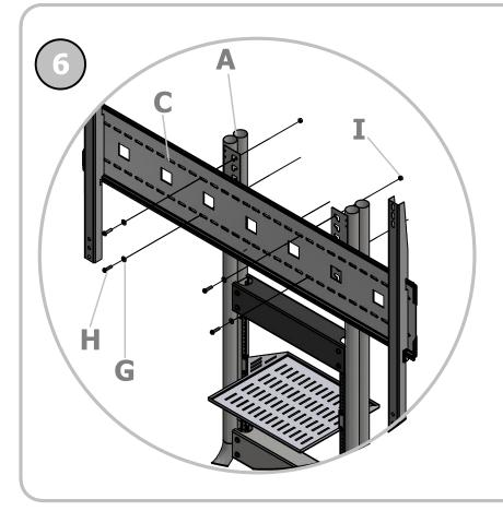
Install the display mount (C) To the cart legs (A) using the hardware indicated
