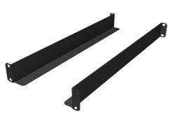
The 6" equipment support brackets can be cantilever mounted at the rear of any Mighty Mo rack and used to support equipment mounted to the front rails. Deeper equipment support brackets are sized to the 16-1/4" to 30" channel racks and 4-point mount with the equipment's mounting ears to provide zero unit support from front to back.
