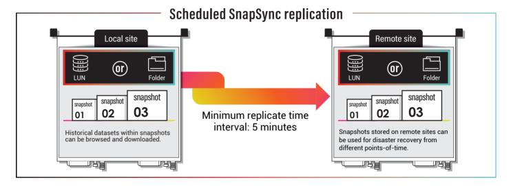
SnapSync creates either a real-time or a scheduled replication job between two QES systems. Disaster recovery can be performed through remote replication to minimize the impact from site failure, as data can be immediately retrieved from the remote backup site.
