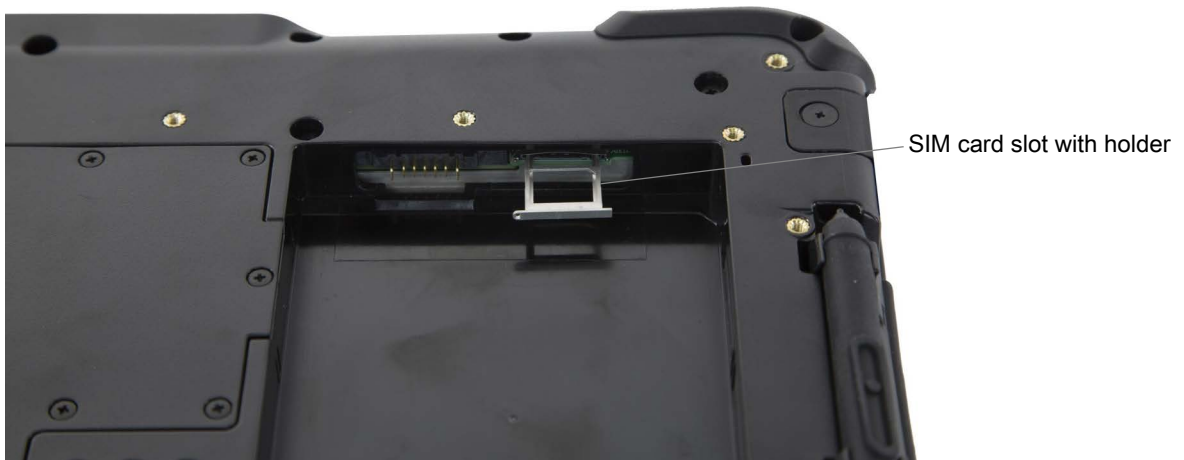
Figure 2 SIM Card Slot with Holder
