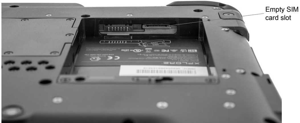
Figure 2 SIM Card Slot with Holder
