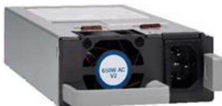
Figure 14. 650W AC power supply (C9K-PWR-650WAC-R)
