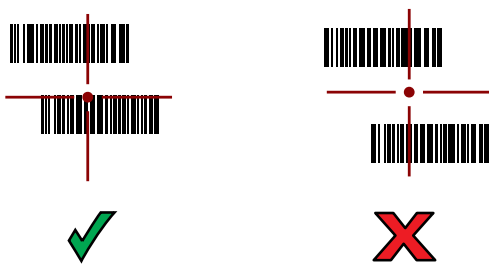
Figure 35 RS5100 Pick List Mode with Multiple Barcodes in Aiming Pattern
