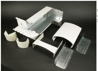
Mounts DS4000 Series Raceway around wall offsets and columns with maximum offset depth of 9'' (229mm). Minimum Offset: 3'' (76mm). Maximum Offset: 9 3/4'' (235mm).
