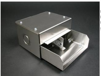
Has concentric 1/2" and 3/4" trade size KOs on end, sides and bottom for feeding S4000 Series Raceway. Use punch kit to increase KO size up to 1 1/4". Removable divider furnished and two No. 10-32 ground terminals provided.
