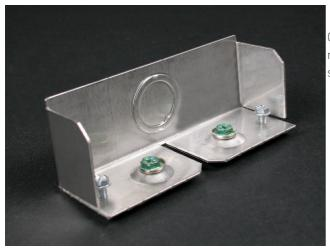
Closes off open end of S4000 Base. Use where one end feed is required in an undivided installation. Includes one 1/2'' - 3/4'' trade size KO and two No. 10-32 ground terminals.
