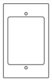
Available in standard width. Provided with bezel to accept up to three (3) dual Wiremold CM Series Open System communication modules or Pass and Seymour Activate Connectivity System inserts. Modules and inserts sold separately.
