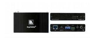
TP-583R is a high-performance, long-reach HDBaseT receiver for 4K HDR HDMI, RS-232 and IR signals over twisted pair. TP-583R converts the HDBaseT signal and outputs it to its HDMI and control ports. It enables extending video signals to up to 70m (230ft) over Kramer copper cables at up to 4K@60Hz (4:4:4) video resolutions. It is compatible with standard HDBaseT-compliant extenders at 4K@30Hz and HD video resolutions
