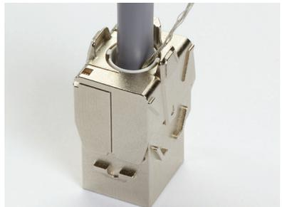
**STEP 6:** Use a cable tie to fix the drain wire cable to the rear shield base body.
