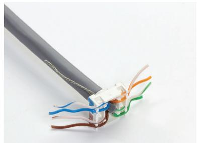
**STEP 3:** After the wires are seated in the 4-pair plastic cap, trim the excess wires along the edge of the cap by using a diagonal cutter.
