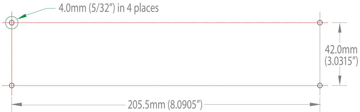
FIGURE 4-3. DIRECT SURFACE MOUNTING MEASUREMENT STENCIL
