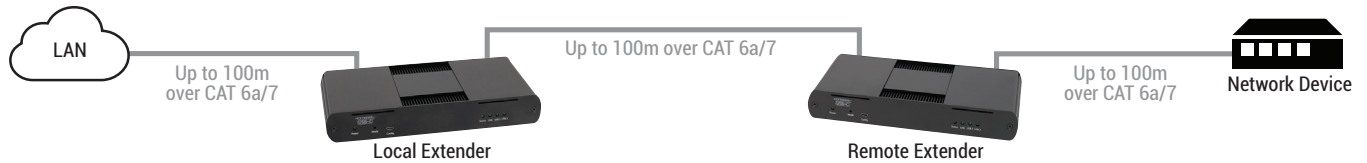
FIGURE 3-2. ETHERNET PASSTHROUGH APPLICATION
