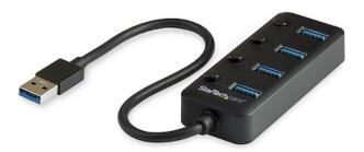
This portable USB 3.0 hub gives you an easy way to add four USB 3.0 Type-A ports to your laptop, with individual power switches to save power. The USB port expander plugs easily into your laptop's USB Type-A port. Plus, it's bus-powered for easy portability.
