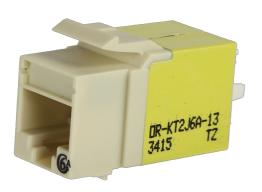
Category 6A Keystone jack, 8-position, 180 degree exit, icon compatible, T568A/B wiring, Elec Ivory, individually packaged. Keystone, KT2J jacks and modules feature New installer friendly lacing cap termination with free termination tool in every carton. The keystone footprint allows flexibility in installation scheduling because its rear insertion into the faceplate allows the technician to complete the termination before and during the construction process.
