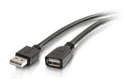
This USB Active Extension cable is an ideal solution for USB applications which require more cable length than the five meter (16.5ft) length limitation of USB. This extension cable actively buffers the incoming and outgoing signals to ensure compliance with USB's 2.0 specification for electrical and timing minimums. The plenum rated jacket meets the requirements for an installation in a commercial space Both low and high speed USB devices will function equally well with this extension.
