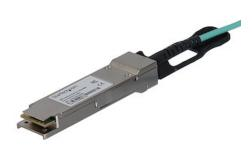
The QSFP40GAO15M is an MSA compliant optical quad small form-factor pluggable (QSFP+) cable that is designed, programmed and tested to work with 40 GbE compatible switches and routers. This AOC QSFP+ cable supports 40 Gigabit Ethernet applications (4 x 10GbE) connected through QSFP+ ports. It is a low-power, low-latency cable that is hot-swappable, making upgrades and replacements seamless by minimizing network disruptions.
