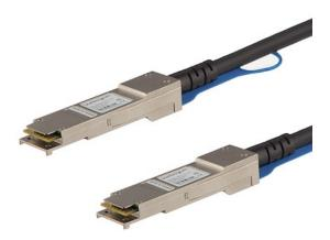
The QSFP40GAC7M is an MSA compliant direct-attach copper QSFP+ cable that's designed, programmed and tested to work in 40G network deployments. It delivers dependable 40 GbE connectivity over copper cabling, which is a cost-effective alternative to fiber-optic cable setups.
