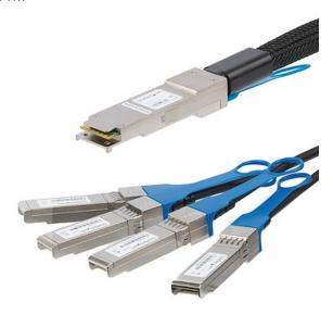
The QSFP4SFPPC1M is an MSA Compliant QSFP+ direct-attach Twinax breakout cable. It is designed, programmed and tested to bridge 40G network equipment with 10G compatible servers or routers. This passive Twin axial cable connects a single QSFP+ port to four 10G SFP+ ports and is fully hot-pluggable making upgrades and replacements seamless by minimizing network disruptions.
