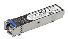
The SFP100BBXUST is an MSA compliant upstream fiber SFP transceiver which pairs with StarTech.com's SFP100BBXDST. They are designed, programmed and tested to work with 100BASE-BX compatible MSA switches and routers. The SFP transceiver module supports a maximum distance of up to 10 km (6.2 mi) and delivers dependable 100 Mbps connectivity over fiber cabling.
