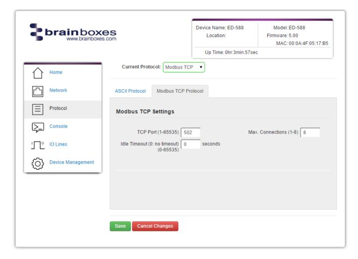
The **TCP port** is a 16 bit number, 1 - 65535, used to identify the services or processes being used in networking communications. Specific port numbers are often used to identify specific services. By convention, TCP port 502 is used by the Modbus protocol.
