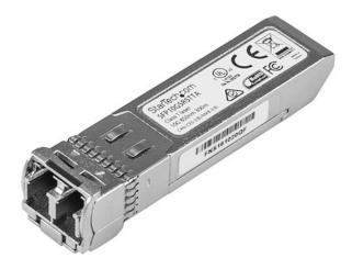
The SFP10GSRST is a TAA compliant Cisco SFP-10G-SR compatible fiber transceiver module that has been designed, programmed and tested to work with Cisco brand switches and routers. It delivers dependable 10GbE connectivity over fiber cable, for 10GBASE-SR compliant networks, with a maximum distance of up to 300 m (984 ft.).
