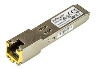
The GLCTSTTAA is a TAA compliant Cisco GLC-T compatible copper transceiver module that has been designed, programmed and tested to work with Cisco brand switches and routers. It delivers dependable 1 GbE connectivity over copper cable, for 1000BASE-T compliant networks, with a maximum distance of up to 100 m (328 ft).
