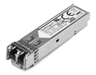
The GLCZXSMRGDST is a Cisco GLC-ZX-SM-RGD compatible fiber transceiver module that has been designed, programmed and tested to work with Cisco brand switches and routers. It delivers dependable 1 GbE connectivity over fiber cable, for 1000BASE-ZX compliant networks, with a maximum distance of up to 70 km (43.5 mi).
