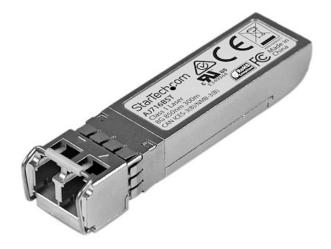
The AJ716BST is an HP AJ716B compatible fiber transceiver module that has been designed, programmed and tested to work with HP brand switches and routers. It delivers dependable 8Gb fiber channel connectivity over fiber cable, for 8GFC compliant networks, with a maximum distance of up to 300 m (984 ft.).
