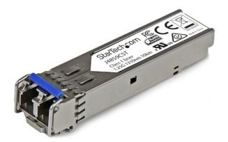
The J4859CST is an HP J4859C compatible fiber transceiver module that has been designed, programmed and tested to work with HP brand switches and routers. It delivers dependable 1 GbE connectivity over fiber cable, for 1000BASE-LX compliant networks, with a maximum distance of up to 10 km (6.2 mi).
