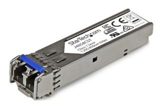
The J4858CST is an HP J4858C compatible fiber transceiver module that has been designed, programmed and tested to work with HP brand switches and routers. It delivers dependable 1 GbE connectivity over fiber cable, for 1000BASE-SX compliant networks, with a maximum distance of up to 550 m (1804 ft).
