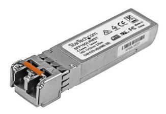
The SFP10GLRMST is a Cisco SFP-10G-LRM compatible fiber transceiver module that has been designed, programmed and tested to work with Cisco brand switches and routers. It delivers dependable 10 GbE connectivity over fiber cable, for 10GBASE-LRM compliant networks, with a maximum distance of up to 200 m (656 ft).
