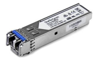
The GLCLHSMDST is a Cisco GLC-LH-SMD compatible fiber transceiver module that has been designed, programmed and tested to work with Cisco brand switches and routers. It delivers dependable 1 GbE connectivity over fiber cable, for 1000BASE-LX/LH compliant networks, with a maximum distance of up to 10 km (6.2 mi).
