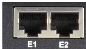
Figure 3-61. Plug expansion boards into these ports.
