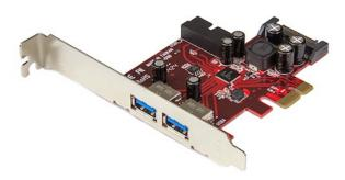
This PCI Express USB 3.0 card offers a cost-effective upgrade that lets you add four USB 3.0 ports to your computer through a PCIe slot. It offers two external ports plus two internal USB 3.0 headers to help adapt your desktop or server to support a variety of USB 3.0 devices.
