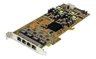
The ST4000PEXPSE 4-Port PoE NIC lets you add four Gigabit Power over Ethernet ports through a single PCI Express slot. Each port can provide up to 25.5W of power, combining network data and power over a single Ethernet cable for reduced cable clutter and added convenience for remote PoE devices.
