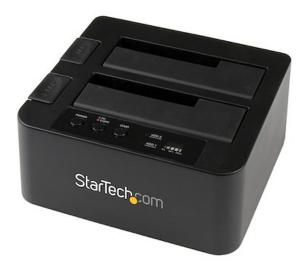
The SDOCK2U33RE Dual 2.5/3.5" SATA HDD/SSD duplicator dock lets you duplicate/clone an existing hard drive without the use of a host computer system -- or dock and swap drives from your desktop or laptop computer simultaneously, using a single USB or eSATA port.
