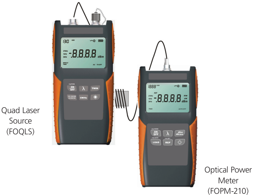
Figure 5-12. Optical power meter (part number FOPM-210) connected to the Quad Laser Source (FOQLS).
