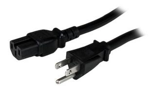
The PXT515C158 8-foot Computer Power Cord features a C15 connector rated for high-temperature equipment, as well as 14 AWG wire suitable for high power connections - a reliable solution for connecting to NEMA 5-15P Power Distribution Units (PDU) located in switchgear rooms and data center environments, or large server applications that require a higher rated, heavier gauge cable.
