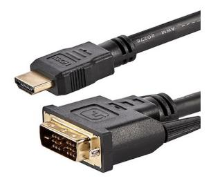
The HDMIDVIMM6 6-foot HDMI to DVI-D cable enables you to connect a DVI-D video card (or other DVI-D output device) to a display that incorporates HDMI technology; the cable supports bi-directional operation that also allows the reverse configuration, delivering digital video from an HDMI-enabled output to a DVI-D capable display.
