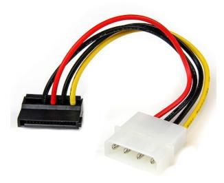
The SATAPOWADPL LP4 to 90-degree SATA power adapter features one 4-Pin LP4 male connector and a left angle, 90-degree SATA power connector (female), which enables you to power a Serial ATA hard drive from a conventional LP4 connection and eliminates the need to upgrade the computer power supply for compatibility with the SATA hard drive.
