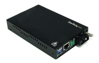
The ET90110SM302 10/100 Mbps Single Mode Fiber Media Converter SC (30 km) lets you extend a Fast Ethernet network (10/100) over single mode fiber, at distances up to 30 km (18.6 miles).
