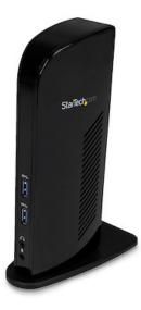
This USB 3.0 dock combines a 6 port USB 2.0/USB 3.0 hub, headphone and microphone audio connectors, and a Gigabit Ethernet RJ45 port into a single docking station.
