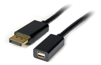
The DP2MDPMF3 3ft DisplayPort to Mini DisplayPort 1.2 Cable Adapter turns a Mini DP male connector into a regular DisplayPort male connector, making it easy to connect a Mini DisplayPort-equipped monitor to a laptop that only provides a standard DisplayPort output (e.g. Toshiba etc.).
