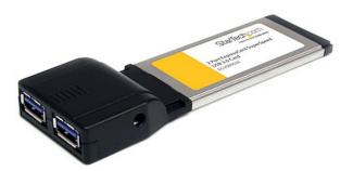
The ECUSB3S22 2-Port ExpressCard USB 3.0 Card adds 2 SuperSpeed USB 3.0 ports to an ExpressCard-enabled computer system, using a 34mm form factor that will fit in both 34mm and 54mm slots, along with ports mounted side-by-side for easy access.
