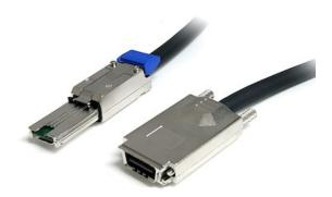
The ISAS88702 2-meter Serial Attached SCSI Cable is designed for high-performance networks, servers, workstations and desktops. This SAS cable features a SFF-8470 (Infiniband) connector and a SFF-8088 (external mini-SAS) connector that supports data transfer rates up to 6 Gbps.
